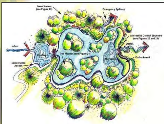
Constructed wetland typical section and plan views DCR Stormwater Design Spec No. 13
