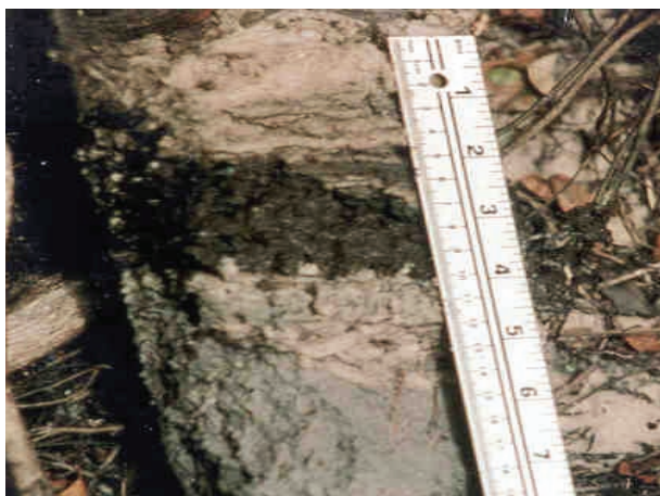
Figure 10. Stratified layers in loamy material.
