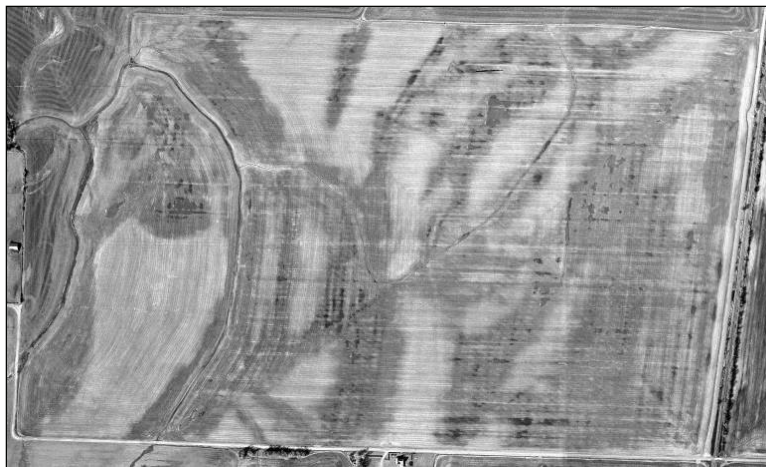
Figure 60. Aerial photograph of an agricultural field with saturated soils indicated by darker colors.
