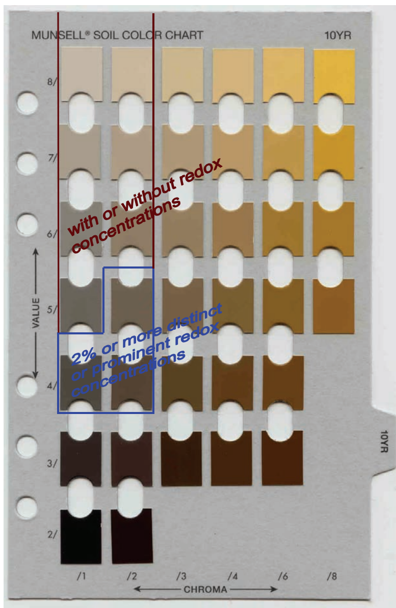
Figure A1. Illustration of values and chromas that require 2 percent or more distinct or prominent redox concentrations and those that do not, for hue 10YR, to meet the definition of a depleted matrix. Due to inaccurate color reproduction, do not use this page to determine soil colors in the field. Background image from the Munsell Soil Color Charts reprinted courtesy of Munsell Color Services Lab, a part of X-Rite, Inc. (Gretag/Macbeth 2000).
