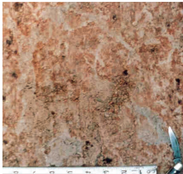
Figure 28. Iron-manganese masses (black spots) in a 40 percent depleted matrix. Scale is in inches.
