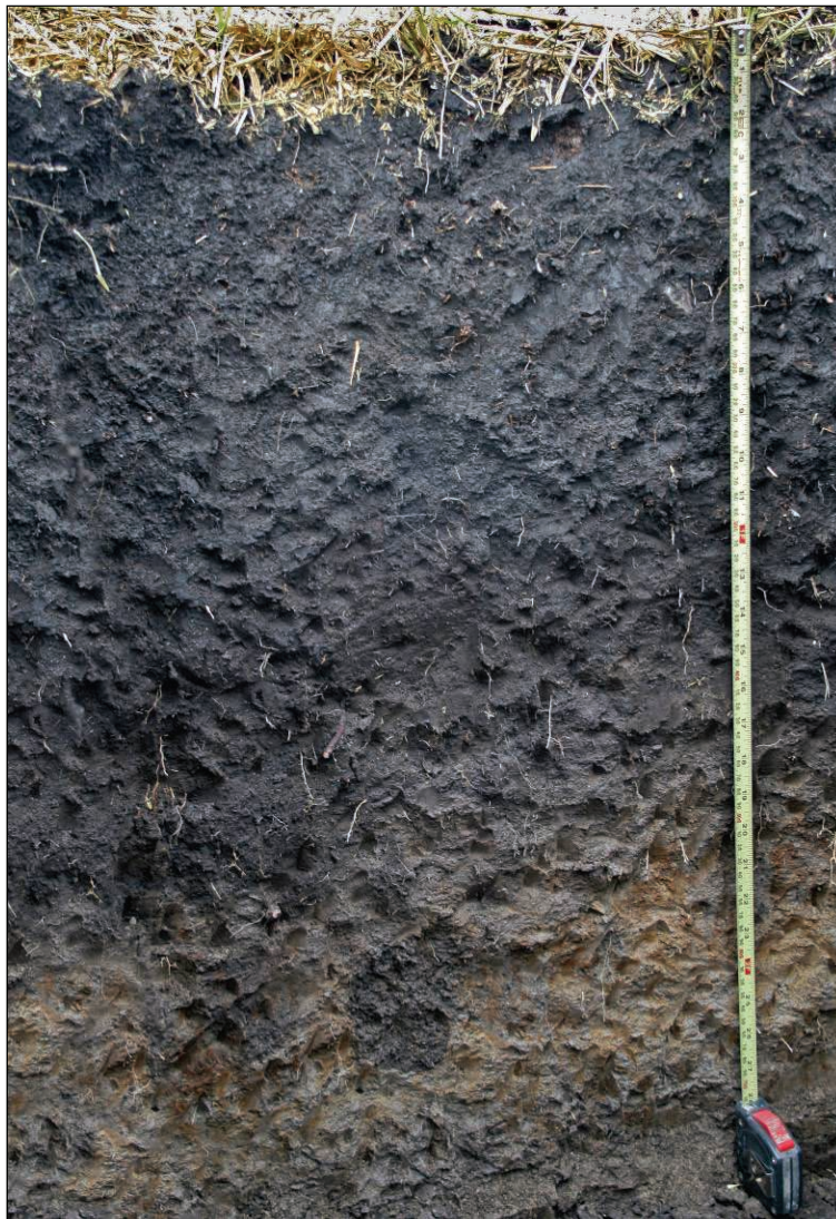
Figure 14. Deep observations may be necessary to identify the depleted or gleyed matrix below a thick, dark surface layer. In this example, the depleted matrix starts at 20 in. (50 cm).
