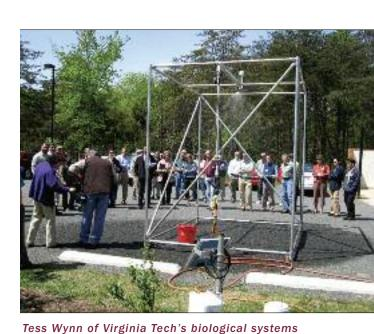
engineer department and Mike Rolband (WSSI) demonstrate the effectiveness of the geogrid pervious parking area with Virginia Tech's rain simulator operating at four inches per hour rate.
